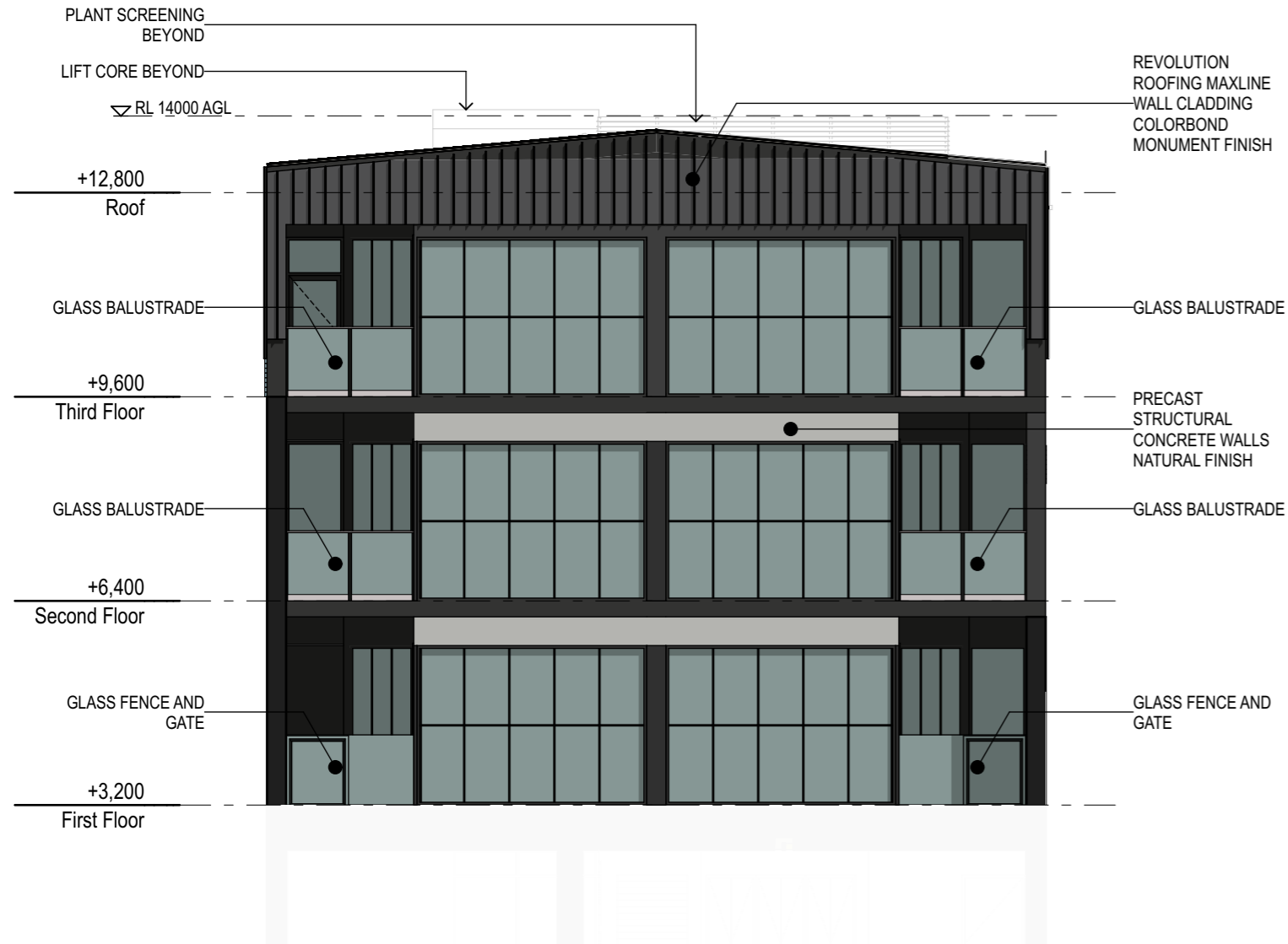
INTERNAL COURTYARD NORTH ELEVATION Scale 1:100
